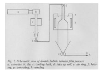
By using an extruder (L/D=25) with the diameter of 115mm as well as a circular die with the diameter 300mm and lip clearance of 1 mm, non-stretched film for large scale production machine was produced at the condition of the resin temperature 265 , blow-up ratio of 1.1, and with a water-cooling ring having the diameter of 330mm.
