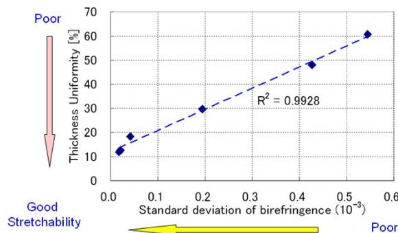
FIGURE 4 Relationship between standard deviation of birefringence distribution and thickness uniformity
