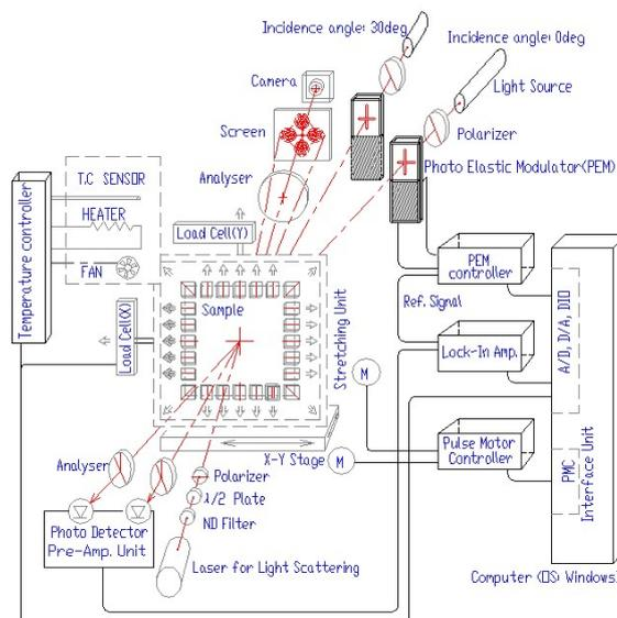
FIGURE 1 A diagram of a newly developed test machine
